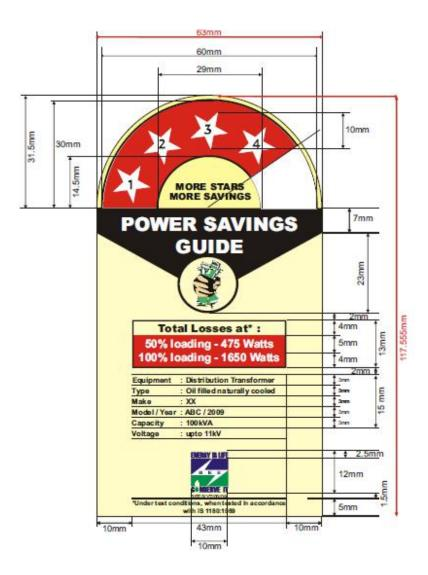
Fig. 3. Colour Scheme: Sample Picture of manner of affixing of Label:
